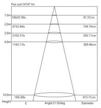
Note:The Curves indicate the illuminated area and the averag illunination when the luminaire is at different distance.
